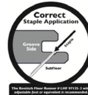
**Note:** Always use a pneumatic flooring stapler that engages the top of the flooring profile over the bottom groove edge at the appropriate angle. Make sure that the flooring stapler is in good working condition and fully seats the staples properly against the bottom groove to prevent top edge or surface damage.
