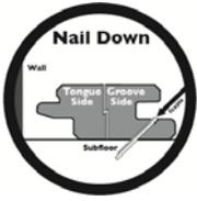
**SPECIAL NOTE: THE PLANK ORIENTATION FOR THE EPIC HARDWOOD 3/8" PRODUCT IS REVERSED FOR THE NAIL DOWN INSTALLATION PROCESS. THE PLANKS WILL BE PLACED WITH THE TONGUES FACING TOWARD THE STARTING WALL. STAPLES WILL BE PLACED THROUGH THE BOTTOM GROOVE EDGE OF THE PLANKS.**
