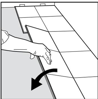
**[8]** Connect the planks in the following rows by aligning the end seam of each plank directly above the end seam of the preceding plank. Insert the long side seam at a slight angle first, and as the top surfaces meet, rotate the plank down into the locked position.
