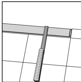
**[10]** For the last row of planks in the room (and perhaps also the first row if you have elected to cut the starting row to a narrower width), cut the panels lengthwise and glue the short ends. (Remember to carefully remove the plastic locking clips before cutting the planks lengthwise!)
