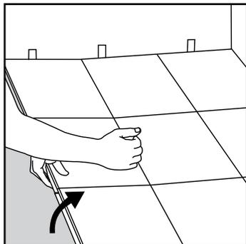
**[1]** Separate the whole row by carefully lifting up and releasing the whole row. Fold up and release the whole long side of the row, being very careful not to allow the planks to bend downward at the end seams! This could damage the locking mechanism of the plank!
