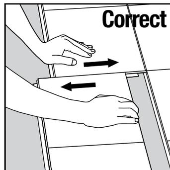
**[2]** Disassemble the panels by sliding them apart horizontally at the end seams. **(Do not fold connected planks upwards!)**
