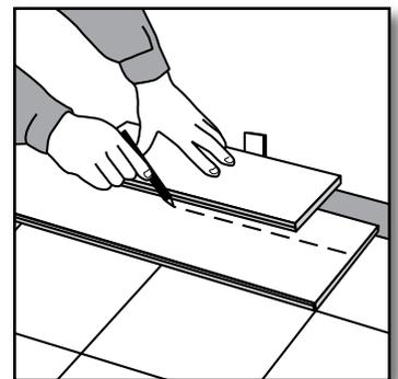
**[11]** Use a full width scrap plank to mark your cutting line on the last row.
