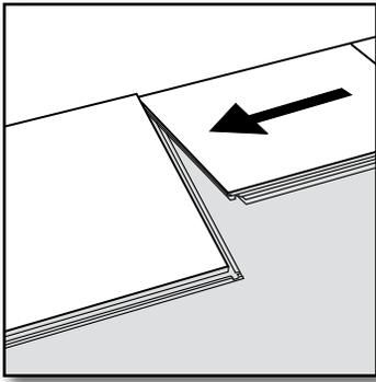
**[2]** In the first row, place the second plank tight against the short end of the first plank.
