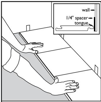
**[1]** Begin the installation in the left-hand corner. Place the plank a minimum of 1/4" from the left wall. Use the installation spacers throughout all perimeter areas to insure the correct expansion space is maintained.
