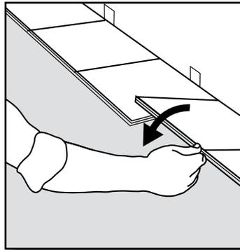
**[3]** Fold down into the locked position with a single movement. The plastic clips will engage to lock this plank into place.
