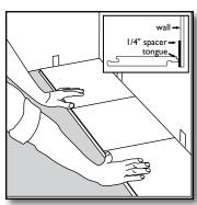
[1] Begin the installation in the left-hand corner. Place the plank a minimum of 1/4" from the left wall. Use the installation spacers throughout all perimeter areas to insure the correct expansion space is maintained.
